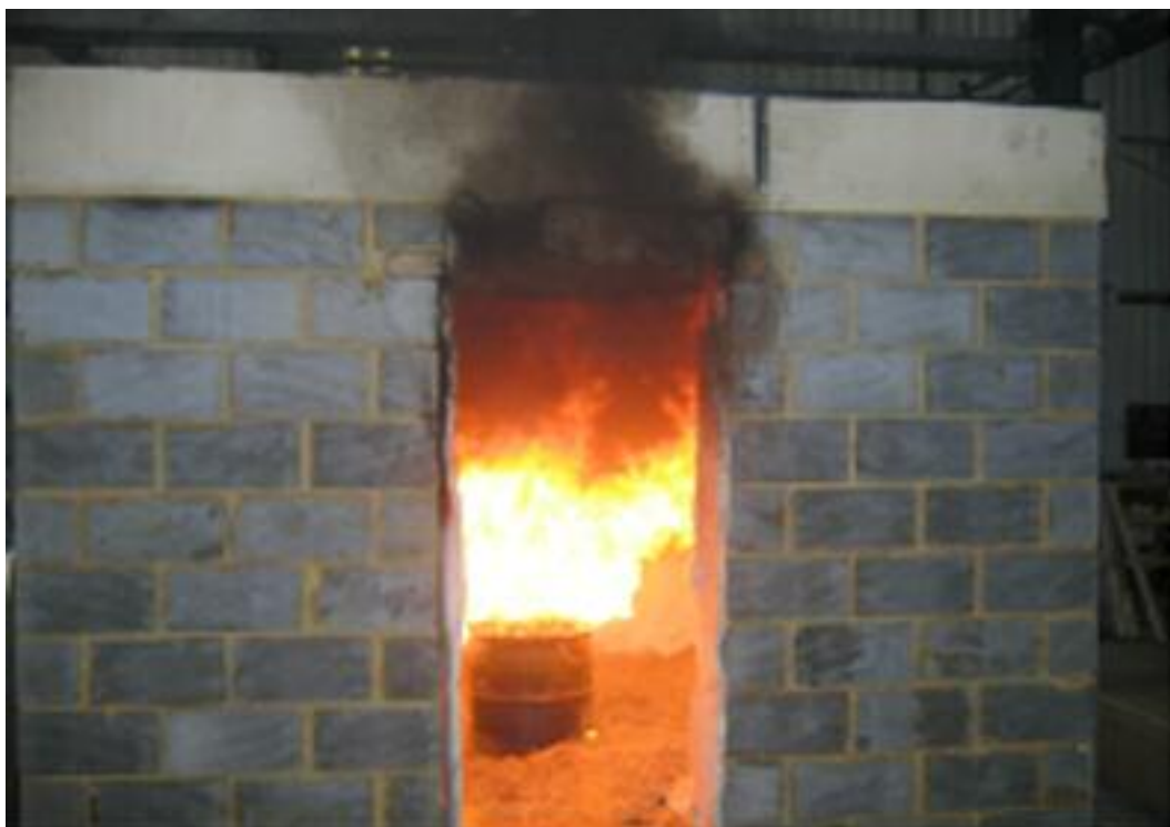
Figure 1: Compartment fire test
