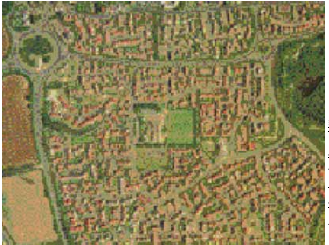
Typical suburban housing 1990's style with houses arranged around a road network designed for the car. Layouts such as this use land inefficiently and make viable public transport almost impossible
