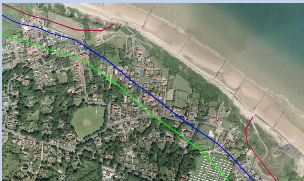
Overstrand 20, 50 and 100 year erosion lines from SMP2. Image courtesy of North Norfolk District Council
