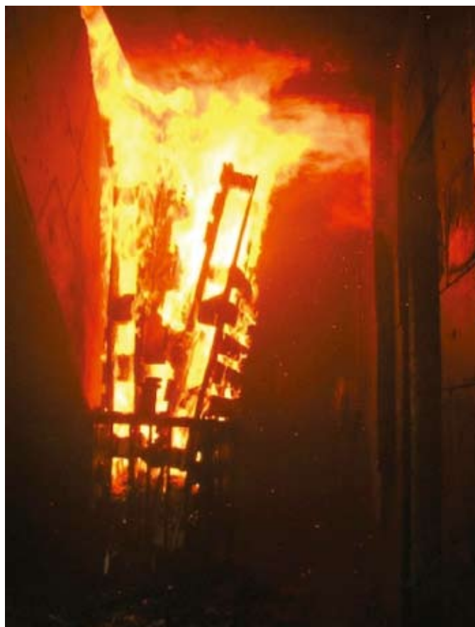
Figure 3.2. An example of a standard FSC crib burning in the Domestic building
